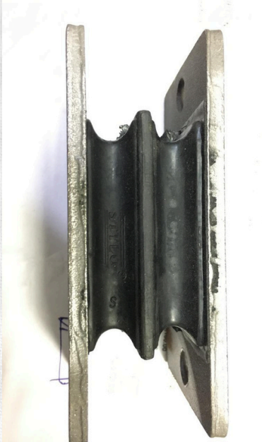
Leyland engine mountin for state transport
